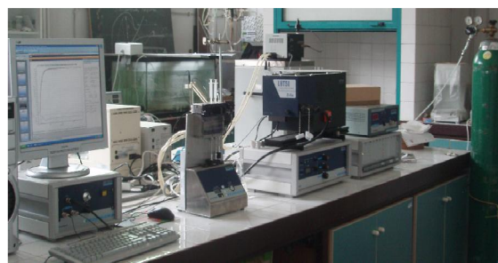
Fig. 3. The stopped-flow equipment set-up
